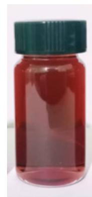
Figure 3: Lignin nanoparticles dispersed in aqueous solution
